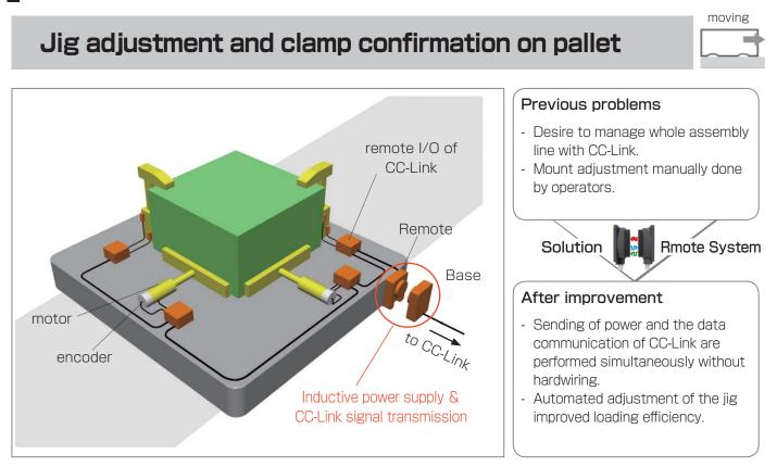
ApplicationControl a Motor, an encoder, a solenoid valve and a sensor installed on the pallet. Utilizing<br/>Field BUS CC-Link.<br/>Remote System sends power to CC-Link remote I/O on a pallet and transmits CC-Link data.
