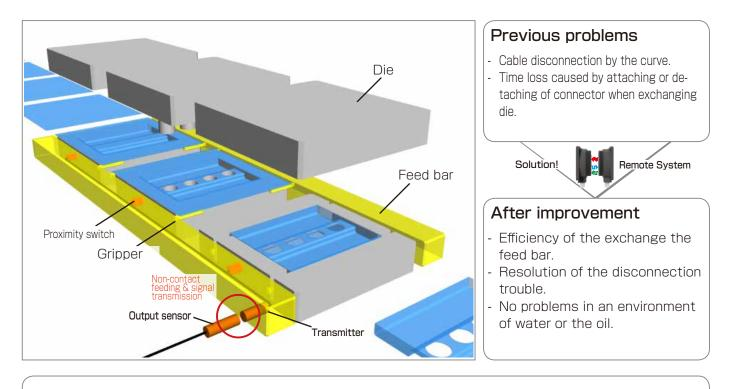
PointBecause of a kind and the placement of the gripper vary according to the press line<br/>using the feed bar, in the case of die exchange the feed bar changes as well. Because<br/>of the remote system the exchange work can be shortened.
