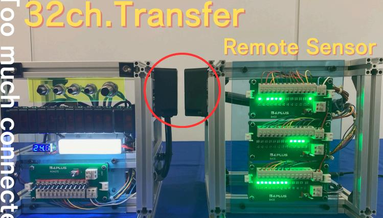
Wireless Power Supply 24VDC/1A +32ch. Signal Transfer (Input)
