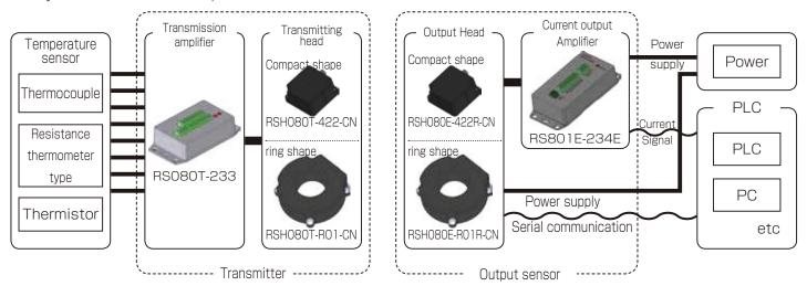
A transmission head and the output head have two kinds of the compact shape and ring geometry. Please choose upon the usage of the environment.
