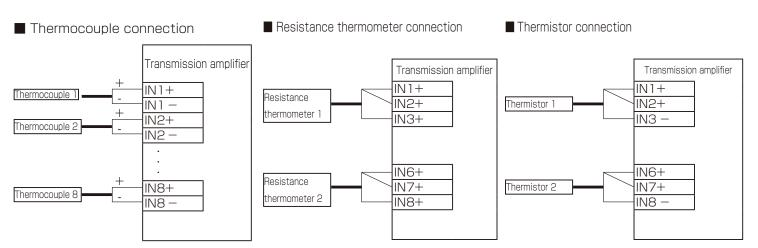
When you connect a thermocouple, place them from IN1, and then connected. When there is a gap between the interval it can cause the disconnection error.
