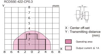
Rated operating distance distance Within 2 mm Shift axis [±4mm] distance 2mm...3mm Shift axis [±1.5mm]
