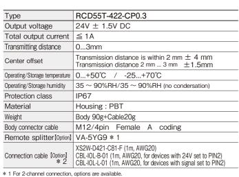
\* 2 The signal of ch 2 is assigned to pin 2 of this system. For chosing the applicable cable, please refer to "connection" on the next page if you connect only 1 ch connecting an IO-Link device with power or signal assigned to pin 2.
