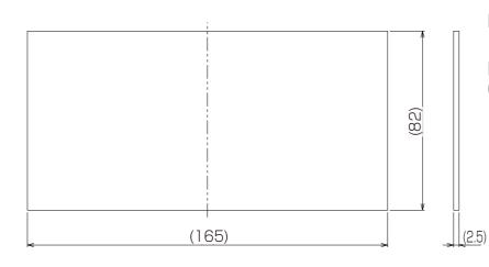
This is a filter that attaches to the inlet part of RCS2000AC (power supply unit). Please use it when replacing the filter.
