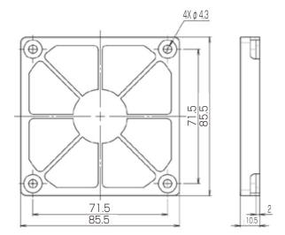
Attached to the intake port of RCS2000AC (power supply unit) A set of guard, special filter, and cover.
